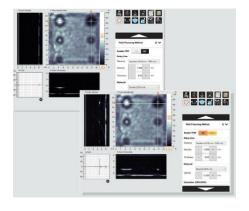
For maximum image quality we also provide Total Focusing Method (TFM) reconstructions, with TFM images available on both vertical and horizontal B-scan views.
