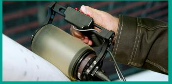
With performance rivaling that of a full immersion C-scan system, our easy-to-use RotoArray gives you faster, more reliable Scan-images, all with the portability of a handheld probe. Together with the Mentor UT, this phased array inspection device allows rapid scanning of a wide variety of materials and components, making ultrasonic inspections even simpler.
