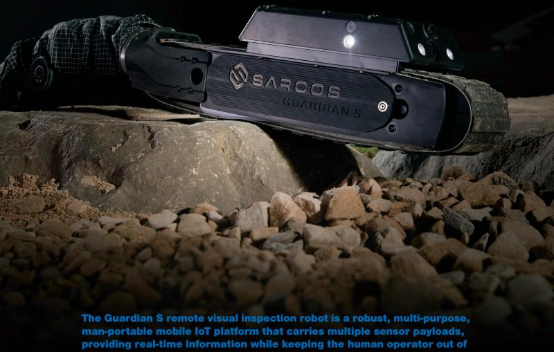
man-portable mobile IoT platform that carries multiple sensor payloads, providing real-time information while keeping the human operator out of harm's way. Optimized for unstructured and unpredictable environments, the Guardian S robot is designed specifically to navigate uneven, challenging terrain and to access small, confined spaces. With the capability for safe teleoperation from remote locations, the Guardian S robot goes where humans either can't or shouldn't go.
